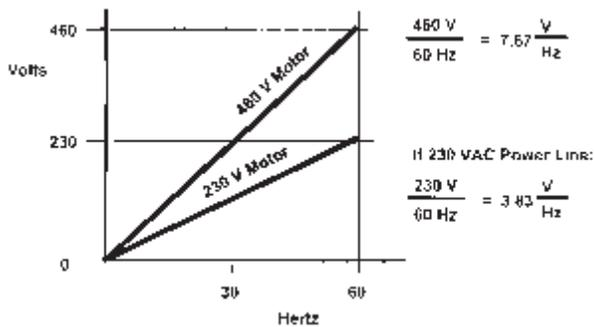
Figure 5, Volts/Hertz Ratio
