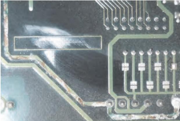
Photo 2, Corrosion on Board Traces Caused by Moisture
