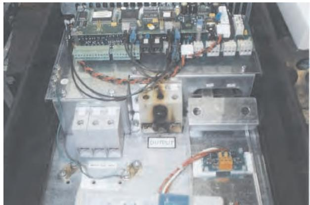
Photo 4, Arcing Caused by Loose Output Contacts
