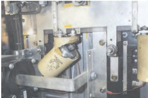
*Photo 6, Capacitor Failure*
